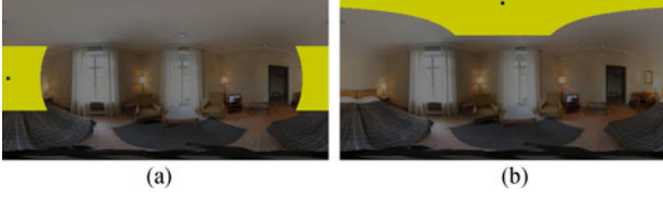
Fig. 3. Local search region when image coordinates fall outside of valid range: the yellow regions represent the local search region and the black points are superpixel centers. Note that the resolution of spherical image is 256 by 512 pixels and search region size is set as 50 pixels for illustration purpose.
