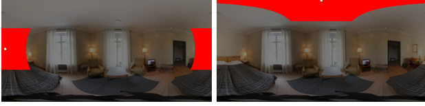
Fig. 2. Local search region (in red) when image coordinates fall outside valid range: the yellow points are superpixel centers. For this 512 \times 256 spherical image, the search region size is set as 50 pixels for illustration purpose.
